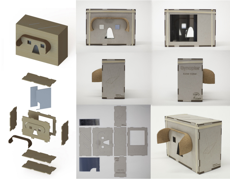
Figure 6: The left column shows renderings of the model, including an ‘exploded view’. The middle and right columns show photographs of the synopter used in this research.
